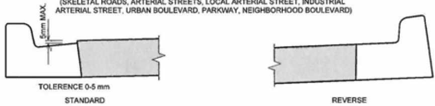
THICKNESS OF ASPHALT CONCRETE TO CURB
