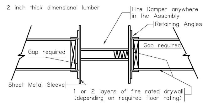
It has been queried whether the detail below is also acceptable, since doubts were expressed about the ability of I-joists to support the drywall and the damper in a fire situation as well as sawn lumber. (The only difference is that the sawn lumber sections have been replaced by engineered joists)
